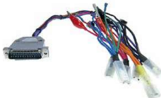
1.9 A wiring harness for ignition module testing (RM02):
