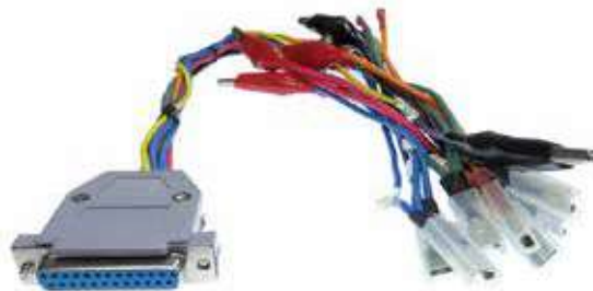
1.8. A wiring harness for regulator testing (RM01):
