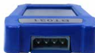
Fig. 2. Connector for diagnostic cable.
